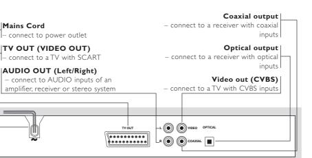
Caution: Do not touch the inner pins of the sockets on the rear panel. Electrostatic discharge may cause permanent damage to the unit.
